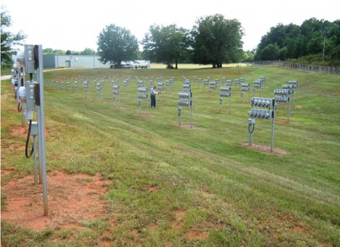
Figure 12-1 Measurements of aggregate maximum and average RF fields found along two rows of Smart Meters in the Itron meter farm during normal operation of the meters.
