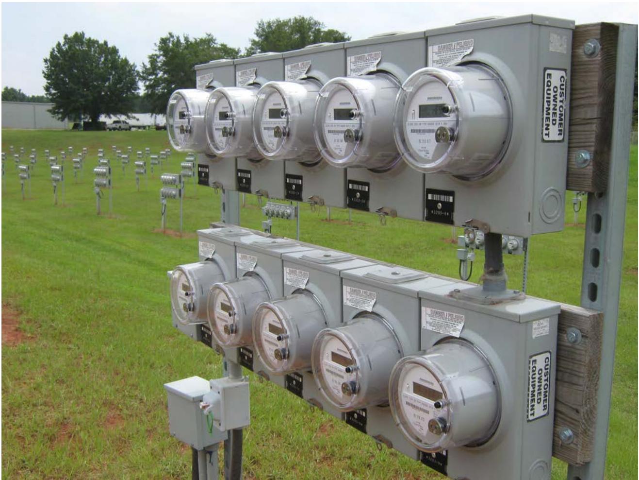
Figure 9-2 Typical rack of ten meters shown in the western part of the Itron meter farm.
