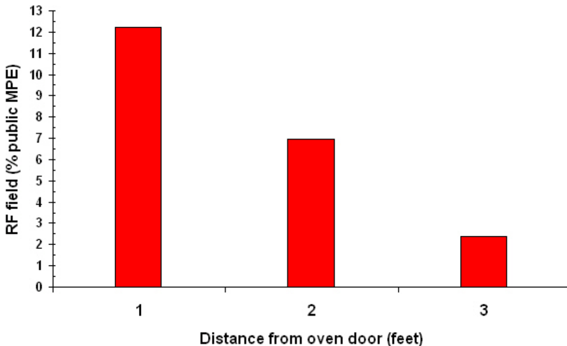
Figure 13-2 Microwave oven leakage vs. distance.
