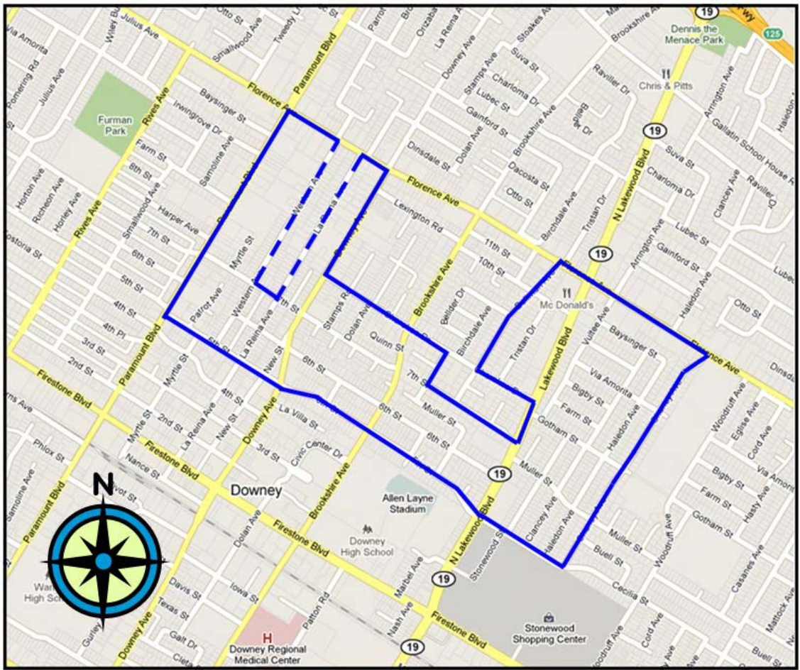
Figure 9-25 Route in Downey, CA neighborhood with SCE deployed Smart Meters over which a driving survey was conducted to test the ability to detect RF signals associated with residential meter installations.
