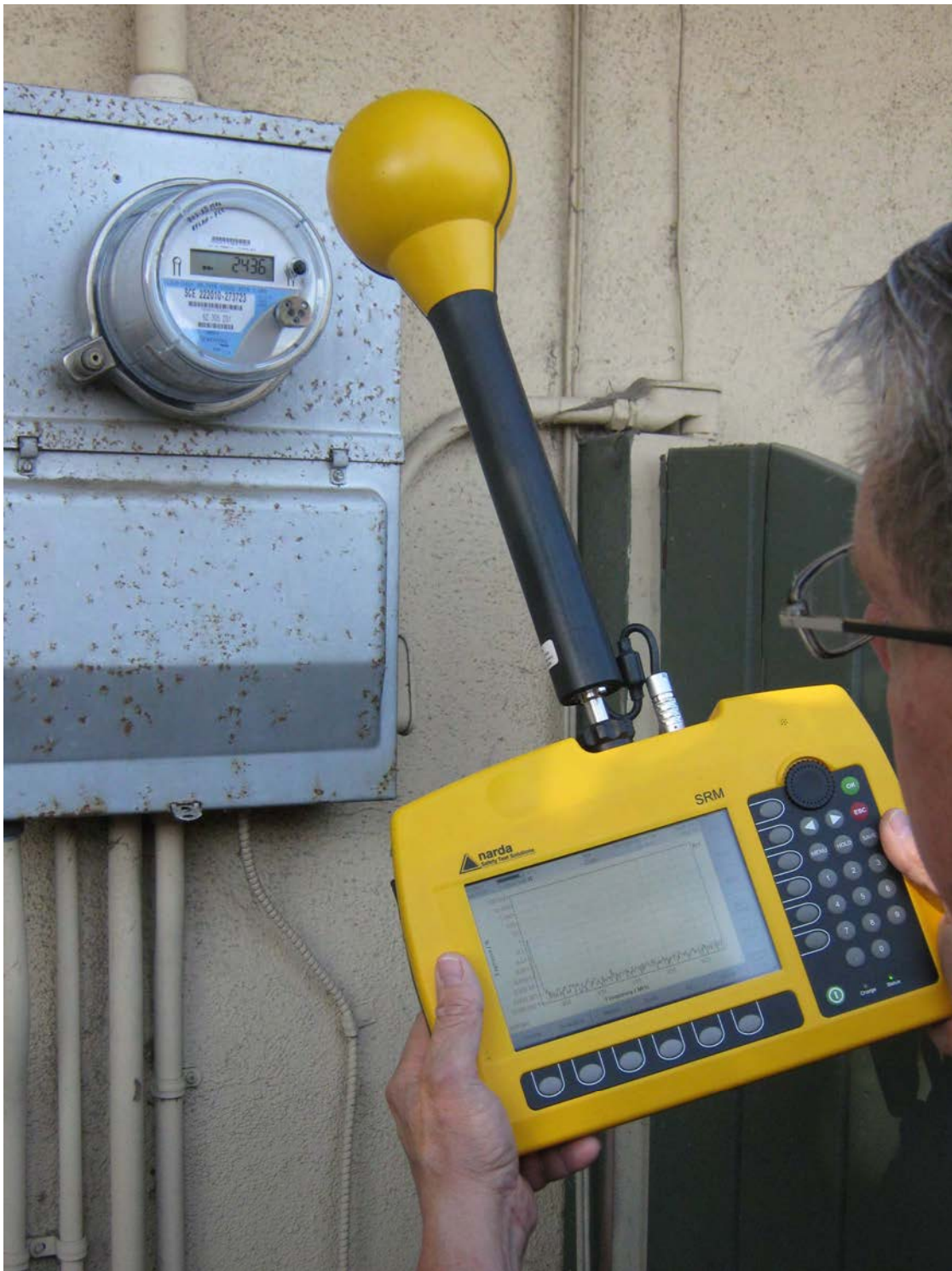
Figure 9-14 Planar scans were performed at several distances in front of a residential Smart Meter by slowly moving the SRM-3006 within a plane at a fixed distance.
