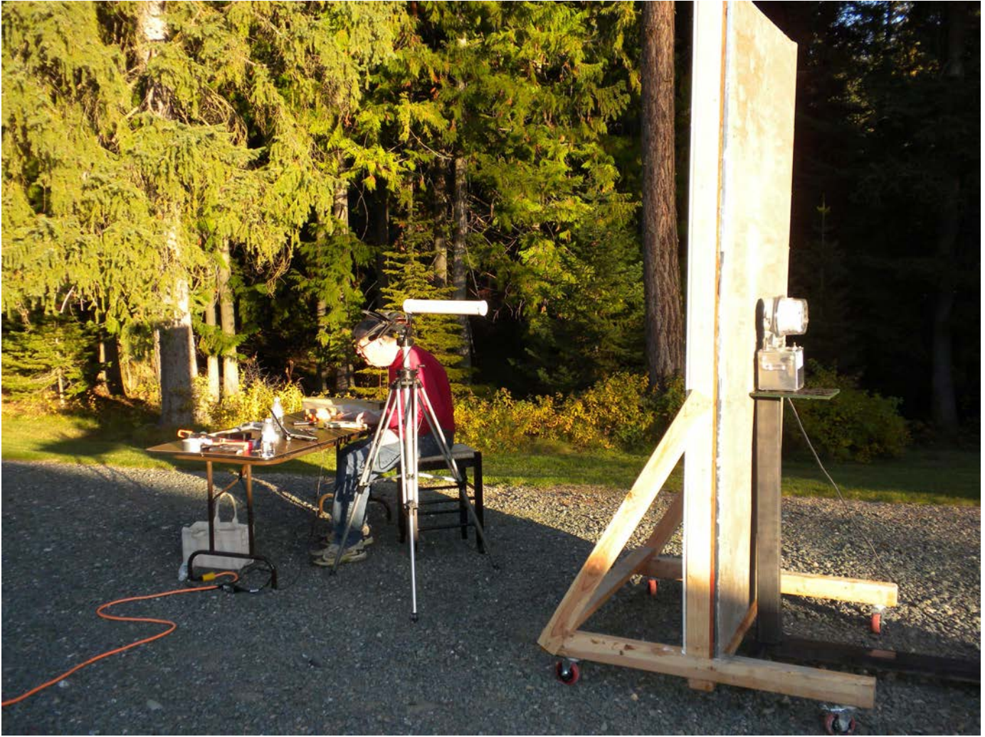
Figure 10-5 Measurement setup for determining insertion loss of simulate stucco wall shown with the 2.4 GHz yagi antenna.
